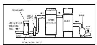
**A CAUTION** Damage to the heater or filter may result if concentrated chlorine is allowed to flow through them.
