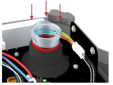
Gently lower the quartz tube into the unit until the Oring makes contact with the top of the black threaded sealing sleeve. Then place the aluminum compression washer and gasket on the quartz tube. Press down on the aluminum compression washer with an even steady pressure. Lift aluminum washer and check to make sure it is seated evenly around the circumference of the quartz tube. Replace aluminum washer.
