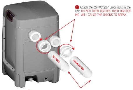
**2** After cutting pipes to length, debur all cut pipe to ensure shavings don't plug critical points internal to the unit. Use PVC solvent cement to glue pipes into the union sleeve. NOTE the inlet and outlet pipe positions.
