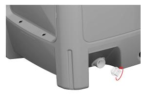
Remove Winterizing O-ring plug near the bottom of the unit. Note, there will be an initial rush of water from the unit after the plug is removed. Allow unit to completely drain, this will take 1-2 minutes. Re-install O-ring plug hand tight.
