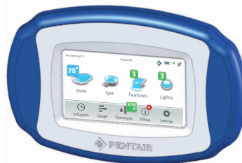
IntelliCenter Control System Wireless Control Panel (P/N 522036)
